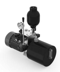
Engineered to complete the braking system and make it more efficient, safe and suitable for the specific application. All power units have redundant return valves, oil temperature control system and hand operated system to be used in case of power failure. The units are available for both oil-applied and spring-applied hydraulic brakes.
